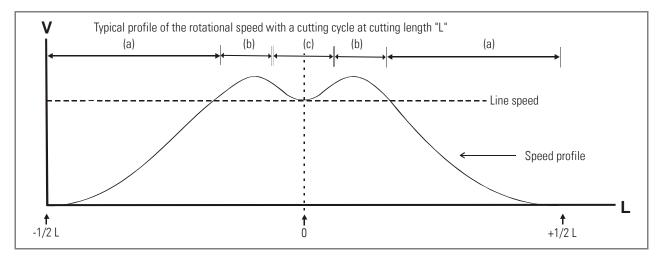
Zone (a) results from the ratio between the cutting length and the active rotating circumference of the tool.
