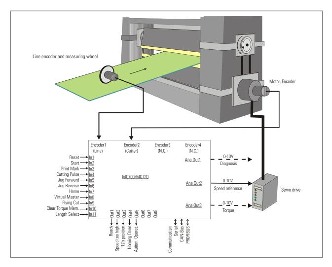
These cutting systems require the horizontal speed of the cutting tool to be synchronous to the material at any time of the penetration of the tool, whereas outside of the penetration zone, it is the cutting length and the active radius of the rotation that determine the speed profile.
