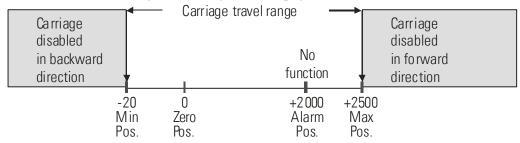
Input Start/Stop = High, automatic cutting cycle or immediate cut:
