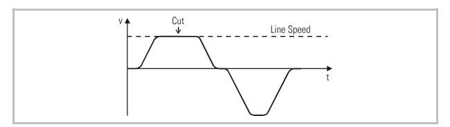
The FS340 or FS641 controller continuously measures the line speed and calculates an anticipation value to start the carriage before the cutting length is reached. Thus the shear will exactly match the cutting position of the material upon completion of the acceleration ramp and no overshoot or oscillation will take place prior to the cut. This saves time and increases the cutting efficiency of the shear system considerably.
