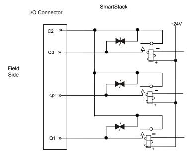
Specification for transient voltage suppressors (transorbs) used on output circuitry is 400 VDC, bidirectional 400 W.
