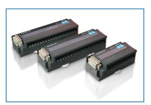
8 DC inputs and 8 relay outputs 8 DC inputs and 8 -.5 amp DC outputs
