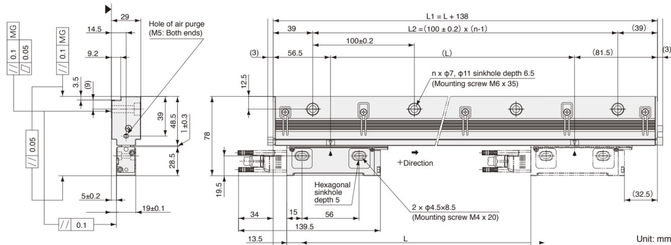
\*When scale head moves in the direction of the arrow, positive polarity is addition and negative polarity is subtraction. \*Cable leadout direction can be selected either right or left.
