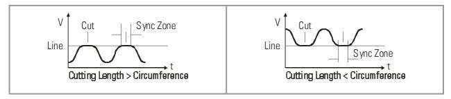
Continuous closed loop control of the relative roll position with respect to the length progress of the line, combined with a short update time provide best cutting accuracy and exceptional smooth motion of the cutting roll at any time.
