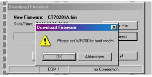
The PC now requests you to set the controller to the "boot mode". To do this, slide the front switch from the "Run" position to the "Program" position and push the Reset button located behind the front plate, by means of a pin
