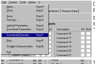
Connect the PC to the controller, using a RS232 cable (see 3.8 of the hardware manual). Apply power to the controller and start the OS5.0 PC software. Select "Download Firmware" from the "File" menu.
