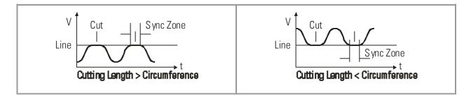
Continuous closed loop control of the relative roll position with respect to the length progress of the line, combined with a short update time provide best cutting accuracy and exceptional smooth motion of the cutting roll at any time.
