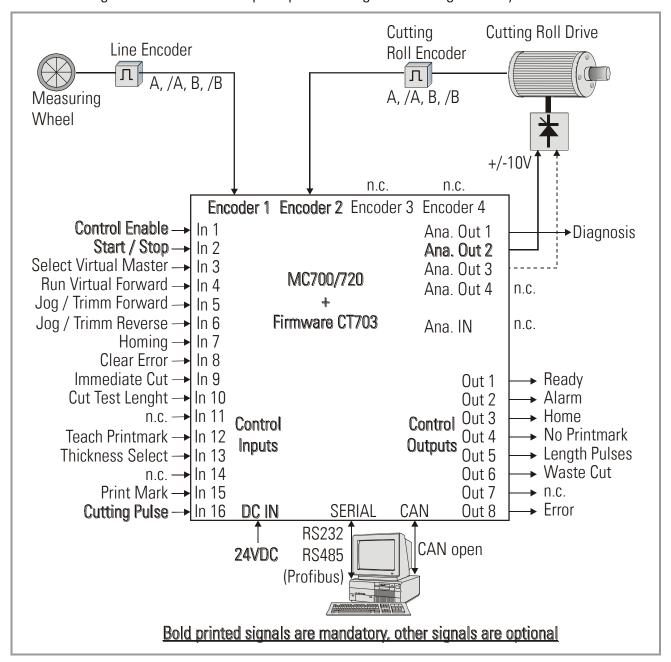
The line encoder must be connected to input "Encoder 1" and the cutting roll encoder to input "Encoder 2".
