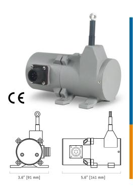
The PT8510 can operate from an unregulated 14.5 to 40 VDC power supply while providing an output signal that is proportional to the linear movement of its measuring cable. The PT8510 has a maximum measurement range up to 60" and has 4 output signal options to choose from: 0...10, 0...5, -10...+10 and -5...+5 Vdc.
