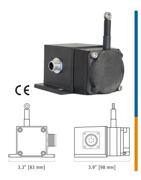
The PT1MA adds 4...20 mA position feedback signal to Celesco's compact line of cable-extension transducers. The PT1MA is available with full stroke ranges from as little as 2 inches on up to 50 inches with adjustable zero and span settings to precisely match the full scale output to your exact measurement range.
