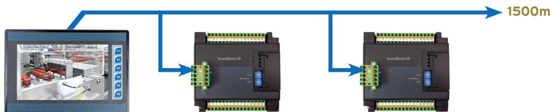
CsCAN supports up to 253 nodes with a maximum network distance of 1500 meters.
