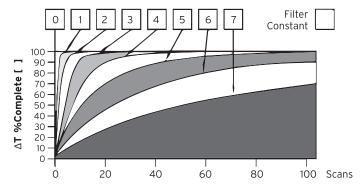
**Digital Filtering:** The illustration above demonstrates the effect of digital filtering (set with Filter Constant) on module response to a temperature change.
