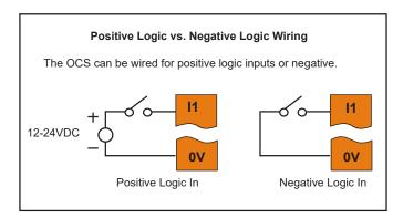
Digital inputs may be wired in either a Positive Logic or Negative Logic fashion as shown. The setting in the Cscape Hardware Configuration for the Digital Inputs must match the wiring used in order for the correct input states to be registered. When used as a normal input and not for high speed functions, the state of the input is reflected in registers %11 - %112.
