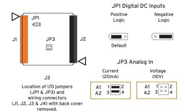
NOTE: The Cscape Module Configuration must match the selected I/O (JP) jumper settings. (Cscape Path: Controller > Hardware Configuration > Local I/O > Config > Module Setup > Analog In)
