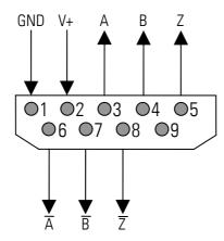
The unit accepts a power supply from 5 to 30 volts, which must be applied to pins 1 and 2 of the connector. The maximum current consumption is about 100 mA. In general, the same power source will be used which normally would also supply the encoder, but also any other remote power source is acceptable.
