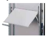
**Description:** Mounted directly to the doorframe it provides a solid surface for documents, computer or measuring devices. The desk can be easily folded and locked within the doorframe space. An automatic safety positioning system locks the desk at angles of 55, 70 and 90 degrees. The DDK 800 can also be mounted on a 1000 mm wide door, by the use of the DCP 1000 accessory.
