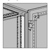
**Description:** To achieve 19", or partial 19" in 800 mm, wide enclosures, these profiles can be mounted with the mounting brackets DNB or DNC. To achieve 19" in 600 mm, wide enclosures, use the brackets DND.
