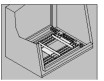
**Description:** In combination with TS supports, to clamp monitor in position.
