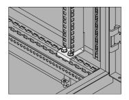
Description: For fixing 482.6 mm, mounting brackets (19") in 600 mm, wide enclosures. Adjustable in depth in 12.5 mm, steps.Material: 3 mm zinc plated steel plate.Pack. quantity: 4 brackets with mounting material.
