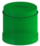
Continuous light element, with integrated LED, green, 230 V AC, Diameter 70 mm
