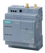
LOGO! CMR2020 communication module for connection LOGO! 8 to GSM/GPRS network; 1 RJ45 port for Ind. Ethernet connection to LOGO! 8; 2xDI; 2xDO; write/read access to LOGO! variables; SMS dispatch/ receiving of text messages; email dispatch; position detection GPS; time synchronization/ forwarding with real time clock; Configuration/diagnostics via web interface; Remote access via OpenVPN/HTTPs, DynDNS; Observe national approval! Manual available as a download.
