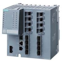
SCALANCE XM408-8C; managed modular IE switch; 8x 10/100/1000 Mbit/s RJ45; 8x 100/1000 Mbit/s SFP; contains 8 combo ports; in total 8 ports can be used; expandable to 24 ports electrical or optical; assembly: DIN rail/S7 mounting rail, PROFINET IO device; redundancy functions; office features (RSTP, VLAN, IGMP,...); C-PLUG in scope of supply; layer 3 integrated.
