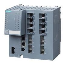
SCALANCE XM408-4C; managed modular IE switch; 8x 10/100/1000 Mbit/s RJ45; 4x 100/1000 Mbps ST-/SC- pluggable as combo ports; in total 8 ports can be used; expandable to 24 ports electrical or optical; assembly: DIN rail/S7 mounting rail, PROFINET IO device; redundancy functions; office features (RSTP, VLAN, IGMP,..); C-PLUG in scope of supply; layer 3 integrated.
