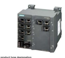
SCALANCE X310, managed plus IE switch, 3x 10/100/1000 Mbit/ and 7x 10/100 Mbit/s RJ45 ports LED diagnostics, error signaling Contact with select/set pushbutton, PROFINET IO device, network management, Integrated redundancy manager, office features (RSTP, VLAN, IGMP,...) C-plug in scope of supply.
