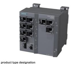
SCALANCE X310FE, managed plus IE switch, 10x 10/100 Mbit/s RJ45 ports, LED diagnostics, error-signaling contact with Select/set pushbutton, PROFINET IO Device, network management, integrated redundancy manager, Office features (RSTP, VLAN, IGMP,...) C-plug in scope of delivery .
