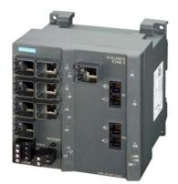
\*\*\*\*\*\*\*\*\* spare part \*\*\*\*\*\*\*\* SCALANCE X308-2, managed plus IE switch, 2x 1000 Mbit/s SC 1x 10/100/1000 Mbit/s and 7x 10/100 Mbit/s RJ45 ports, LED diagnostics, error signaling contact with select/set button, PROFINET IO device, network management, integrated redundancy manager, office features (RSTP, VLAN, IGMP,..) C-plug in scope of delivery 30
