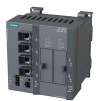
SCALANCE X308-2M TS; managed IE switch, compact; 4x 10/100/1000 Mbit/s for RJ45 ports electrical; 2x 100/1000 Mbit/s for 2-port media modules, electrical or optical; LED diagnostics; error signaling Contact; PROFINET IO device; network management; integrated redundancy manager; Office features (RSTP, VLAN, IGMP,...); C-plug in scope of delivery extended temperature range with railway approval EN 50155;
