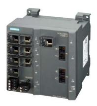
SCALANCE X308-2, managed plus IE switch, 2x 1000 Mbit/s MM SC 1x 10/100/1000 Mbit/s and 7x 10/100 Mbit/s RJ45 ports, LED diagnostics, error signaling contact with select/set pushbutton, PROFINET IO device, network management, integrated redundancy manager, office features (RSTP, VLAN, IGMP,...) C-PLUG in scope of supply.
