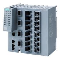
SCALANCE XC216-4C G manageable Layer 2 IE switch; IEC 62443-4-2 certified; Full gigabit; 12x 10/100/1000 Mbps RJ45 ports; 4x 1000 Mbps combo ports (either 1000 Mbps/ SFPs or 10/100/1000 Mbps RJ45 ports can be used); 1x console port; diagnostics LED; redundant power supply; temperature range -40 °C to +70 °C; assembly: DIN rail/S7 mounting rail/wall; redundancy functions; office features (RSTP, VLAN,...); PROFINET IO device; Ethernet/IP-compliant; C-PLUG slot; IEEE 1588v2 PTP
