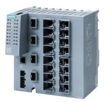
SCALANCE XC216-4C manageable Layer 2 IE switch; IEC 62443-4-2 certified; 12x 10/100 Mbit/s RJ45 ports; 4x 1000 Mbit/s combo ports (either 1000 Mbit/s/ SFPs or 10/100/1000 Mbit/s RJ45 ports can be used); 1x console port; diagnostics LED; redundant power supply; temperature range -40 °C to +70 °C; assembly: DIN rail/S7 mounting rail/wall; redundancy functions; office features (RSTP, VLAN,...); PROFINET IO device; Ethernet/IP-compliant; C-PLUG slot;
