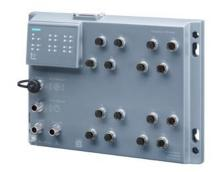
SCALANCE XP216, managed IE switch, 12x 10/100 Mbit/s IEC 62443-4-2 certified; M12 ports, 4x 10/100/1000 Mbit/s M12 ports IP65, LED diagnostics, error signaling contact, redundant power supply, PROFINET IO device, network management, can be operated in redundant ring, incl. dust caps, including electronic manual on CD-ROM, C-PLUG optional.
