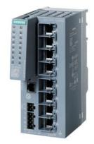
SCALANCE XC208EEC manageable Layer 2 IE switch; IEC 62443-4-2 certified; 8x 10/100 Mbit/s RJ45 ports; 1x console port; diagnostics LED; redundant power supply; with painted printed-circuit boards; NAMUR NE21-compliant; temperature range -40 °C to +70 °C; assembly: DIN rail/S7 mounting rail/wall; redundancy functions; Office; features (RSTP, VLAN,...); PROFINET IO device; Ethernet/IPcompliant; C-PLUG slot;
