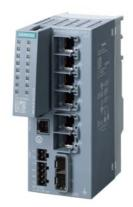
SCALANCE XC206-2SFP G EEC manageable Layer 2 IE switch; IEC 62443-4-2 certified; 6x 10/100/1000 Mbit/s RJ45 ports; 2x 1000 Mbit/s SFP; 1x console port; diagnostics LED; redundant power supply; with painted printed-circuit boards; NAMUR NE21-compliant; temperature range -40 °C to +70 °C; assembly: DIN rail/S7 mounting rail/wall; redundancy functions; office features (RSTP, VLAN,...); PROFINET IO device; Ethernet/IP-compliant; C-PLUG slot;
