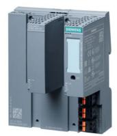
XF204-2BA IRT managed IE IRT switch, 4 x 10/100 Mbit/s, 2 x Bus adapter interface , error signaling contact, with set pushbutton, redundant 24 V DC power supply, PROFINET IO device, network management, Redundancy Manager integrated, incl. electron. manual on CD-ROM, C-PLUG optional.
