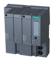
SCALANCE XF204 managed two BusAdapters BA 2xRJ45 HA IEC 62443-4-2 certified; IE switch, 4 x 10/100 Mbps, 2 x BusAdapter interface, error signaling contact, set pushbutton, redundant 24 V DC power supply, PROFINET device, extended temperature range -40 °C...+70 °C, conformal coating, with electronic manual on DVD, C-PLUG optional, delivery with BusAdapter. 6DL1193-6AR00-0AA0
