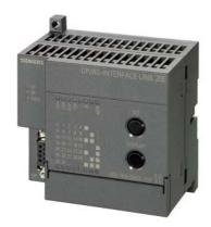
SIMATIC NET, DP/AS-Interface Link 20 E, Gateway PROFIBUS DP/AS-Interface according to AS-Interface specification V 3.0 in degree of protection IP20
