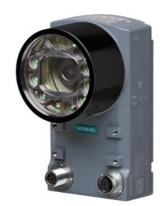
SIMATIC MV530 S optical reader resolution: 800 x 600 pixels; Function: 1D/2D code reading; operating range [mm]: 30...250, depending on dot size; image field[mm]: 40x30...185x140; PoE; IP67; delivery: complete reader incl. built-in ring lamp green, pole filter, Optic 5.6 mm (fix- focus, fixed cover) and protective barrel;
