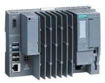
SIMATIC ET 200SP Open Controller, CPU 1515SP PC2, 8 GB RAM (basic device 6ES76772DB400AA0), 128 GB CFast with Windows 10 IoT Enterprise 64-bit and S7-1500 Software Controller CPU 1505SP preinstalled, interfaces: 1x slot CFast, 1x slot SD/MMC, 1x connection for ET 200SP BusAdapter PROFINET, 1x 10/100/1000 Mbps Ethernet, 2x USB 3.0; 2x USB 2.0, 1x DisplayPort, documentation on CFast, restore image on CFast
