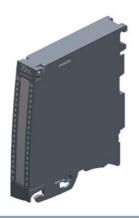
SIMATIC S7-1500, analog output module AQ 2x U/I ST, 16-bit resolution accuracy 0.3%. 2 channels in groups of 2, diagnostics; substitute value; the module supports the safety-oriented shutdown of load groups up to SIL2 according to EN IEC 62061:2021 and Category 2 / PL c according to EN ISO 13849-1:2015. delivery including front connector push-in, infeed element, shield bracket and shield terminal
