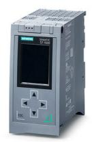
\*\*\*Spare part\*\*\* SIMATIC S7-1500F, CPU 1516F-3 PN/DP, Central processing unit with work memory 1.5 MB for program and 5 MB for data, 1st interface, PROFINET IRT with 2-port switch, 2nd interface, ETHERNET, 3rd interface, PROFIBUS, 10 ns bit performance, SIMATIC Memory Card required
