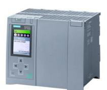
SIMATIC S7-1500T, CPU 1516T-3 PN/DP, central processing unit with work memory 3 MB for program and 7.5 MB for data, 1st interface: PROFINET IRT with 2-port switch, 2nd interface, Ethernet, 3rd interface, PROFIBUS, 6 ns bit performance, SIMATIC Memory Card required
