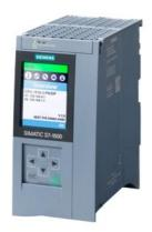
SIMATIC S7-1500, CPU 1516-3 PN/DP, central processing unit with 1 MB work memory for program and 5 MB for data, 1st interface: PROFINET IRT with 2-port switch, 2nd interface: PROFINET RT, 3rd interface: PROFIBUS, 10 ns bit performance, SIMATIC Memory Card required
