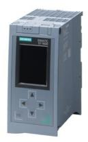
SIMATIC S7-1500R, CPU 1515R-2 PN central processing unit with work memory 500 KB for program and 3 MB for data, 1st interface: PROFINET RT with 2-port switch, 2nd interface: PROFINET, SIMATIC Memory Card required
