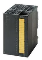
SIMATIC S7, Digital input SM 326, 8 DI; 24 V DC, NAMUR, fail-safe NAMUR input for SIMATIC S7 F-systems, up to Category 4 (EN 954-1)/ SIL3 (IEC61508)/PLE (ISO13849), 1x 40-pole
