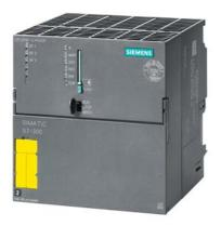
SIMATIC S7-300 CPU319F-3 PN/DP, Central processing unit with 2.5 MB work memory, 1st interface MPI/DP 12 Mbit/s, 2nd interface DP master/slave 3rd interface Ethernet PROFINET, Micro Memory Card required
