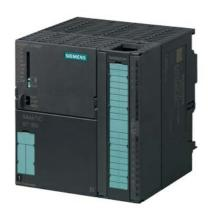
SIMATIC S7-300, CPU 315T-3 PN/DP, Central processing unit for PLC and technology tasks, 384 KB work memory, 1st interface MPI/DP 12 Mbit/s, 2nd interface DP (drive), 3rd interface Ethernet PROFINET with 2-port switch, Integr. I/O for technology, Front connector (1x 40-pole) and Micro Memory Card min. 8 MB required
