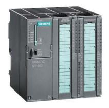
SIMATIC S7-300, CPU 314C-2 PTP Compact CPU with MPI, 24 DI/16 DO, 4 AI, 2 AO, 1 Pt100, 4 high-speed counters (60 kHz), integrated interface RS485, Integr. power supply 24 V DC, work memory 192 KB, Front connector (2x 40-pole) and Micro Memory Card required
