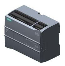
SIMATIC S7-1200, CPU 1215C, compact CPU, AC/DC/relay, 2 PROFINET ports, onboard I/O: 14 DI 24 V DC; 10 DO relay 2 A, 2 AI 0-10 V DC, 2 AO 0-20 mA DC, Power supply: AC 85-264 V AC at 47-63 Hz, Program/data memory 125 KB
