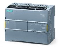
SIMATIC S7-1200F, CPU 1215 FC, compact CPU, DC/DC/DC, 2 PROFINET ports, onboard I/O: 14 DI 24 V DC; 10 DO 24 V DC; 0.5A; 2 AI 0-10 V DC, 2 AO 0-20 mA DC, Power supply: DC 20.4-28.8V DC, Program/data memory 150 KB
