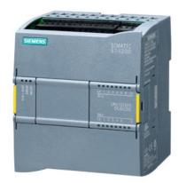
SIMATIC S7-1200F, CPU 1212 FC, compact CPU, DC/DC/DC, onboard I/O: 8 DI 24 V DC; 6 DO 24 V DC; 2 AI 0-10 V DC, Power supply: DC 20.4-28.8V DC, Program/data memory 100 KB
