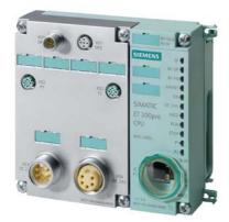
SIMATIC DP, IM154-8 PN/DP CPU f. ET200 PRO, 384 KB work memory, Int. PROFINET interface, Int. PROFIBUS DP master/slave interface Degree of protection IP65/67, Micro Memory Card and Connection module required
