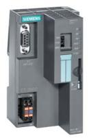
SIMATIC DP, IM151-7 CPU for ET200S, 128 KB work memory with integrated PROFIBUS DP interface (9-pole D-sub socket) as DP slave, without battery SIMATIC MMC required
