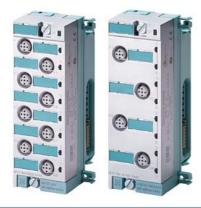
SIMATIC DP, Electronic modules for ET 200 PRO 4 DO 24 V DC, 2.0A High Feature, Channel diagnostics; short-circuit and wire break; incl. bus module, Connection module IO 6ES7194-4..00-0AA0 order separately
