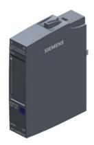
SIMATIC ET 200SP, Analog input module, Al 2x U/l 2-.4-wire High Feat., suitable for BU type A0, A1, Color code CC05, channel diagnostics, 16 bit, +/-0.1%
